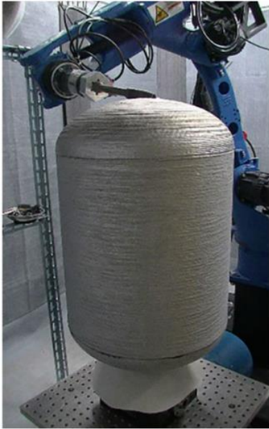
WAAM System (Left) and a Small Tank (40 cm Diameter) Fabricated with WAAM Technology (Right)
