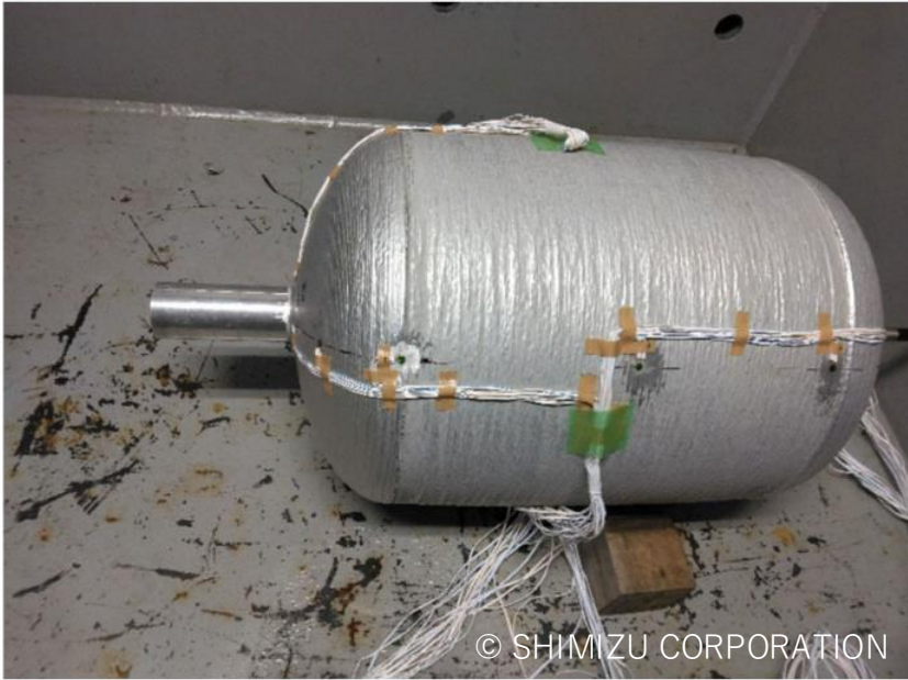
WAAM System (Left) and a Small Tank (40 cm Diameter) Fabricated with WAAM Technology (Right)
